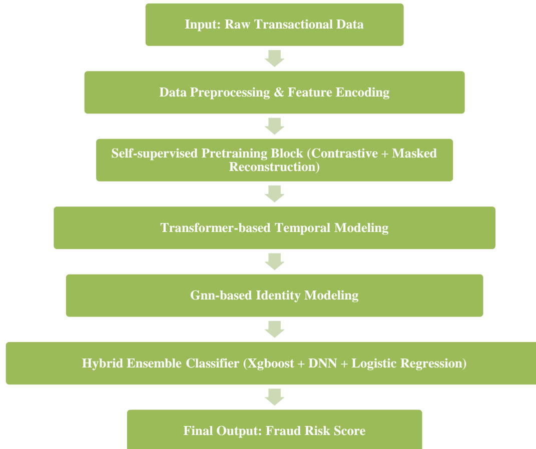
Figure 1: Overall System Architecture Diagram (End-to-End Pipeline)
